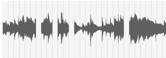
Figure 11. Visual representation of 10% packet loss in a waveform
